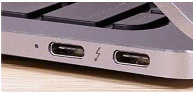
Description: The fastest common connection on the market today, Thunderbolt 3 can transfer data at up to 40 Gbps, four times faster than the fastest USB connection (USB 3.1 gen 2). This high-speed standard can also output to up to two 4K monitors at once, because a single port carries dual DisplayPort signals. On several new devices you can use Thunderbolt 3 to connect to an external graphics card, which allows you to play high-end games on an otherwise slim laptop.
