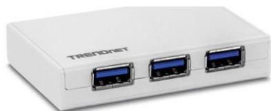
Description: Great for external hard drives, SSDs and high-res docking stations, USB 3.0 has a maximum transfer rate of 5 Gbps, more than 10 times that of its predecessor, USB 2.0. Ports for USB 3 are automatically backward-compatible with USB 2.0 cables and devices.
