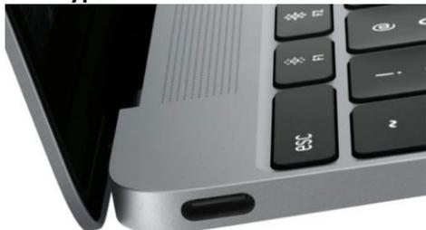
Description: This slim USB port is the connector of the future, already available on a number of devices and likely to replace USB Type-A, USB Type-B and microUSB on all new systems in the near future. Because it's much thinner than its predecessors, Type-C can fit on extremely svelte laptops like the MacBook 12-inch and Asus ZenBook 3. It's also reversible, so you never have to worry about putting your plug in upside down.
