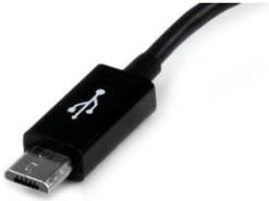
Description: This small port is the charging connector of choice for smartphones and low-power tablets, but you probably won't see it on a laptop or desktop. Regular micro USB ports support USB 2.0 speeds (480 Mbps), but there are a few devices, mostly external hard drives, that have micro USB 3.0 ports which have some extra pins and offer faster transfer rates. You can still use micro USB 2.0 wires and connectors in the micro USB 3.0 ports, however.
