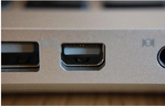
**Description:** DisplayPort is the most advanced display-connection standard today, with the ability to output to a single monitor at 4K resolution and 60 Hz, or up to three monitors at full HD (using a hub or dock). Most laptops that have DisplayPort either use the smaller, mini DisplayPort connector or send their DisplayPort signals out of a USB Type-C port.
